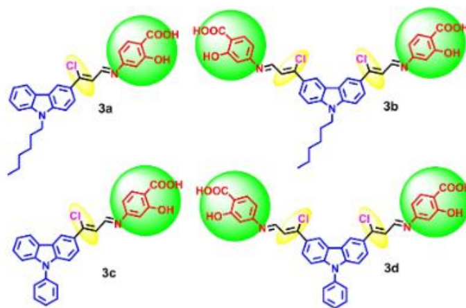
Figure 11. Four those dyes designed and synthesised by Lokhande et al. in 2019 acting as photosensitisers in DSSC
