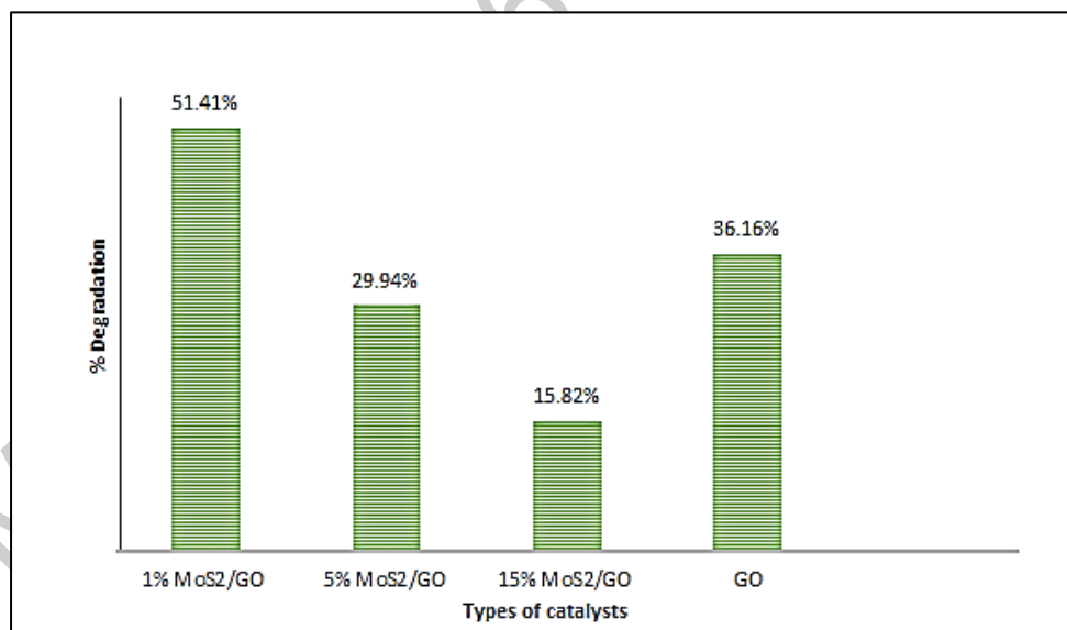
Figure 4. Degradation percentage of 2-chlorophenol for different catalysts under sunlight
