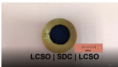
Figure 3. Prepared symmetrical cell LCSO|SDC|LCSO
