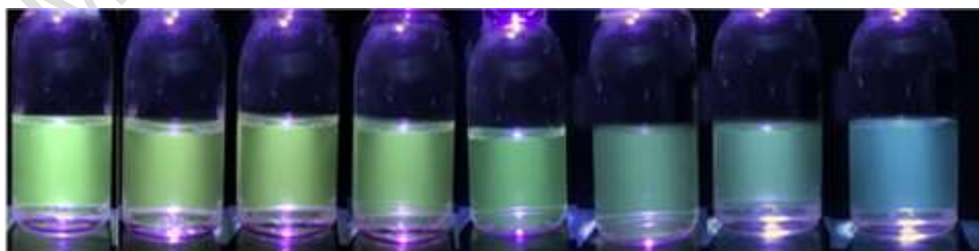
Figure 8. Color progression of h-CQDs with the increasing \text{Hg}^{2+} concentration in simulated seawater
