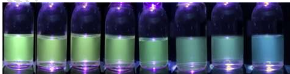
Figure 8. Color progression of h-CQDs with the increasing Hg^{2+} concentration in simulated seawater
