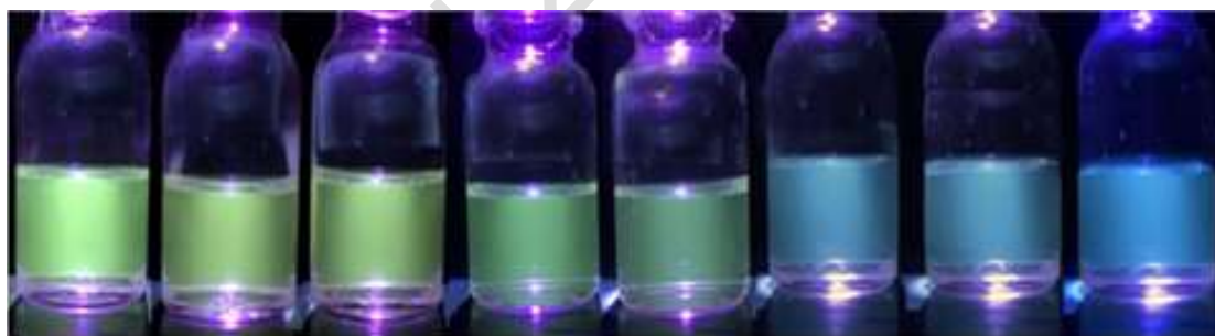
Figure 7. Color progression of h-CQDs with the increasing Hg^{2+} concentration in purified water
