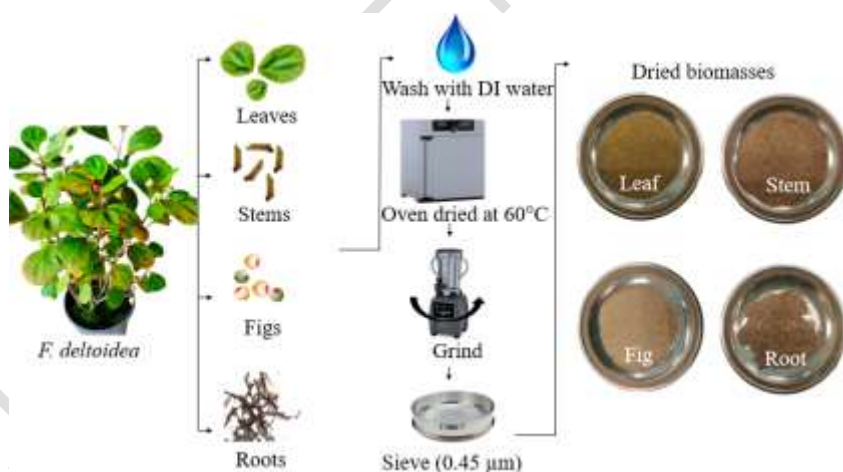
Figure 1. Illustration of the process flow of preparing dried plant biomasses of different organ
