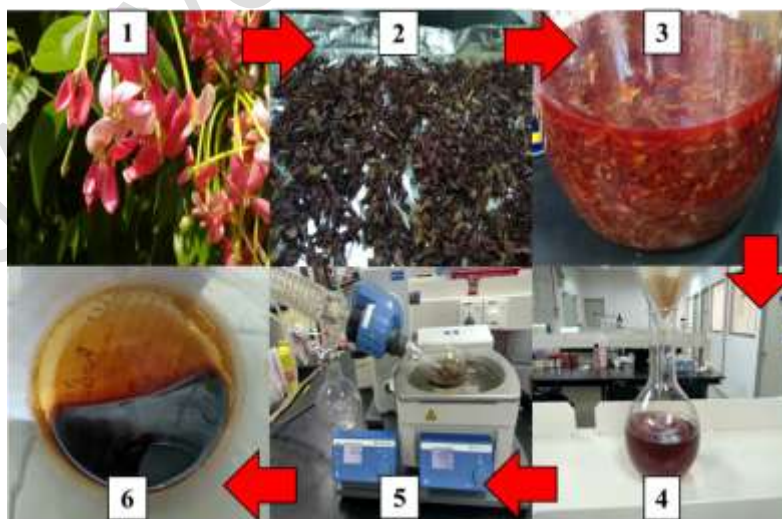
Figure 2. Methanolic dye extract process: (1) raw sample, (2) drying, (3) soaking with methanol, (4) filtered, (5) evaporate to dryness, and (6) dye extract
