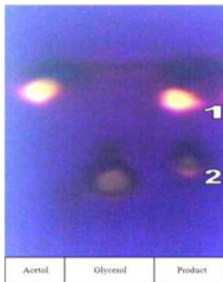
Figure. 1. Thin layer chromatography of commercial sample, glycerol and reaction product (1) acetol; (2) glycerol
