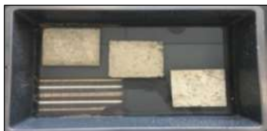
Figure 7. Soaking of slab into the water
