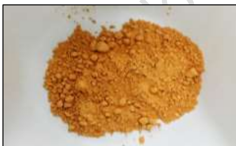
Figure 3. Lead powder used as a reinforcement in concrete
