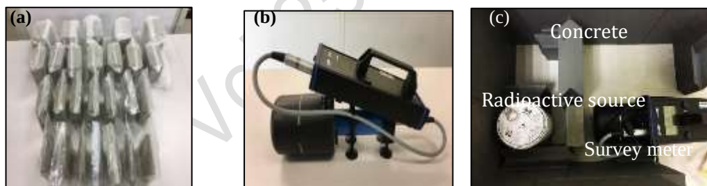
Figure 8. (a) Developed radiation concrete slabs (b) Survey meter (c) Experimental setup in this study
