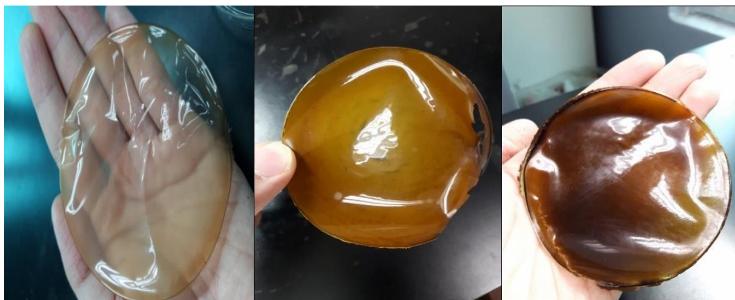
Figure 1. Appearances of chitosan-based films incorporated with different concentrations (0%, 3% and 5% from left to right) of musk lime extracts
