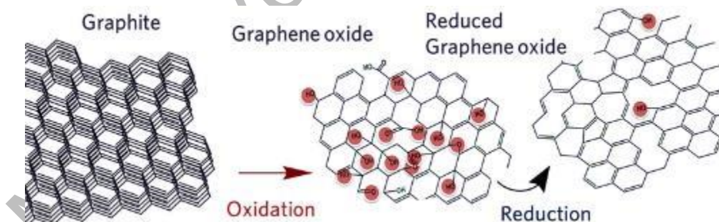
Figure 1. Chemical reaction of graphite to rGO [16]
