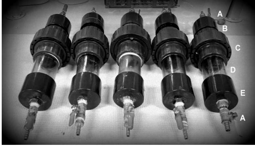
Figure 3. Design of Manganese Oxide cartridges; The brass valves (A), the PVC plug (B), the union with O-ring (C), the clear PVC pipe (D), and the end cap (E)
