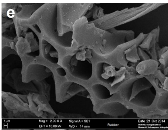
Figure 2. VPSEM of charcoal powder for: (a) Mangrove; (b) commercial charcoal; (c) palm oil; (d) coconut; and (e) rubber tree, using an accelerating voltage of 10 kV
