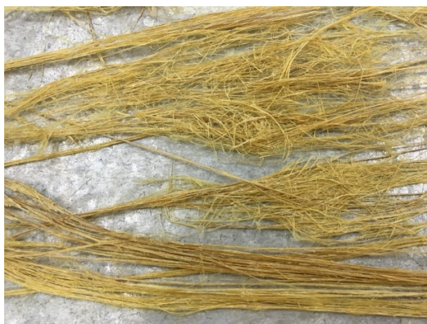
Figure 1. Macroscopic photograph of alkali treated bamboo fibers
