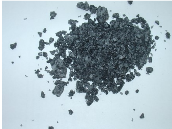
Figure 4. Deactivated Pd/C catalyst taken from the bottom of the reactor
