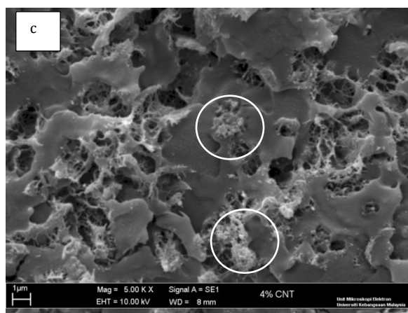
Figure 4. SEM micrograph of a) PLA/LNR at 1.5 wt.% MWCNT b) PLA/LNR at 3.5 wt.% MWCNT and c) PLA/LNR at 4 wt.% MWCNT
