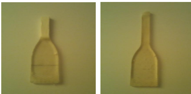
Figure 5. Visualization of deformed samples under tensile test
