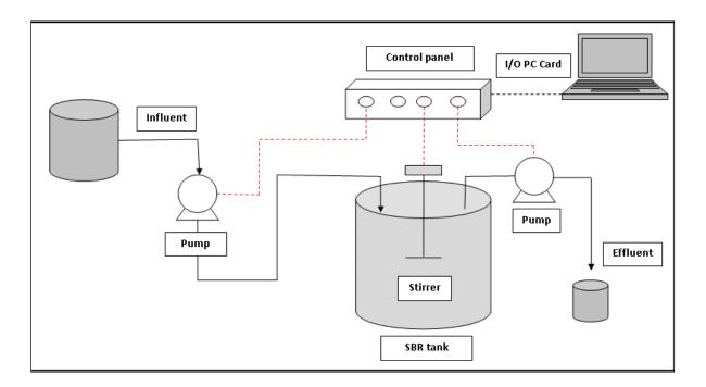
Figure 1. Schematic diagram of SBR system
