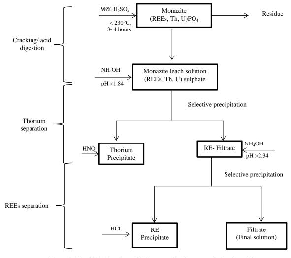
Figure 1. Simplified flowchart of REEs separation from monazite leach solution
