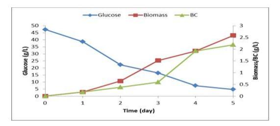
Figure 2. Glucose, biomass and BC profiles when growing *G. xylinus* DSM46604 on 50 g/L glucose media in a 3-L bioreactor.
