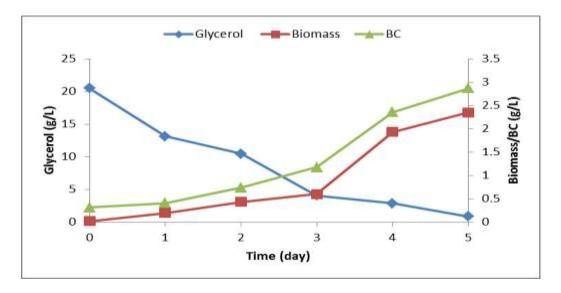
Figure 3. Glycerol, biomass and BC profiles when growing G. xylinus DSM46604 on 20 g/L glycerol in a 3-L bioreactor.
