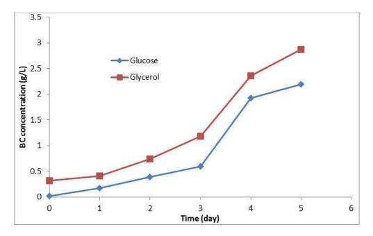
Figure 4. Profile for BC production when growing *G. xylinus* DSM46604 on 50 g/L glucose or 20 g/L glycerol in a 3-L bioreactor
