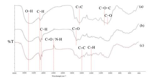
Figure 1. FTIR spectrum for (a) unmodified OPL, (b) modified OPL, and (c) modified OPL after adsorption test with POME
