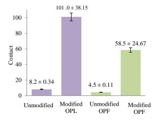
Figure 4. Contact angles for OPL and OPF samples
