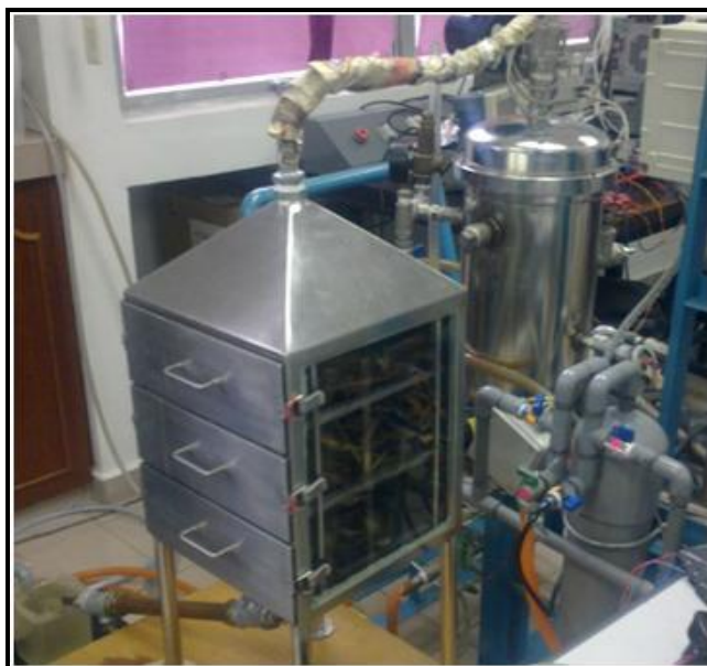
Figure 1. Hydro-diffusion steam distillation system
