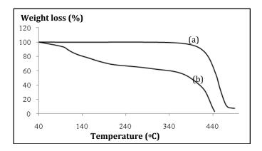
Figure 5: TGA curves of (a) BMI.NTf<sub>2</sub> and (b) BMI.NTf<sub>2</sub>(H<sub>2</sub>SO<sub>4</sub>)
