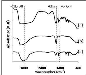
Figure 2: FTIR spectra (a) ChCl, (b) ZnCl<sub>2</sub>, (c) ChCl 2ZnCl<sub>2</sub>
