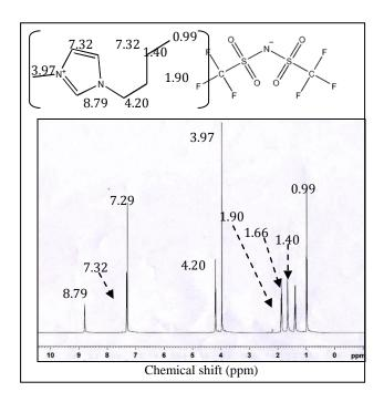
Figure 3. <sup>1</sup>H NMR spectrum of BMI.NTf<sub>2</sub>
