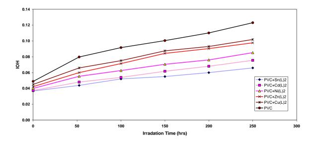
Fig. 4: The relationship between the hydroxyl index and irradiation time for PVC films (30 μm thickness). Containing different additives, concentration of additives are fixed at 0.5% by weight.
