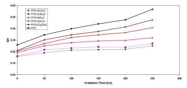
Fig. 3: The relationship between the polyene index and irradiation time for PVC films (30 μm thickness). Containing different additives, concentration of additives are fixed at 0.5% by weight.
