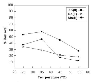
Figure 4: Effect of temperature on metal ion removal on maize stalks
