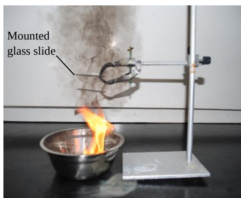
Figure 1: Experimental set-up of control burning in laboratory experiment
