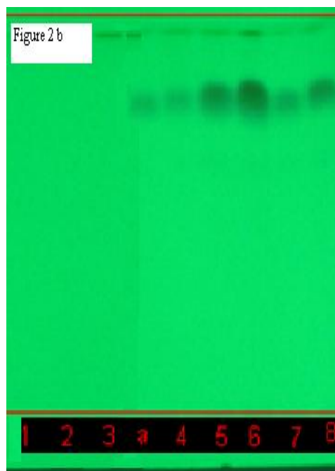
Figures 2a and 2b: HPTLC profile of different fractions (1-8) of flash chromatography and standard mitragynine (a) under UV 365 and UV 254 nm.
